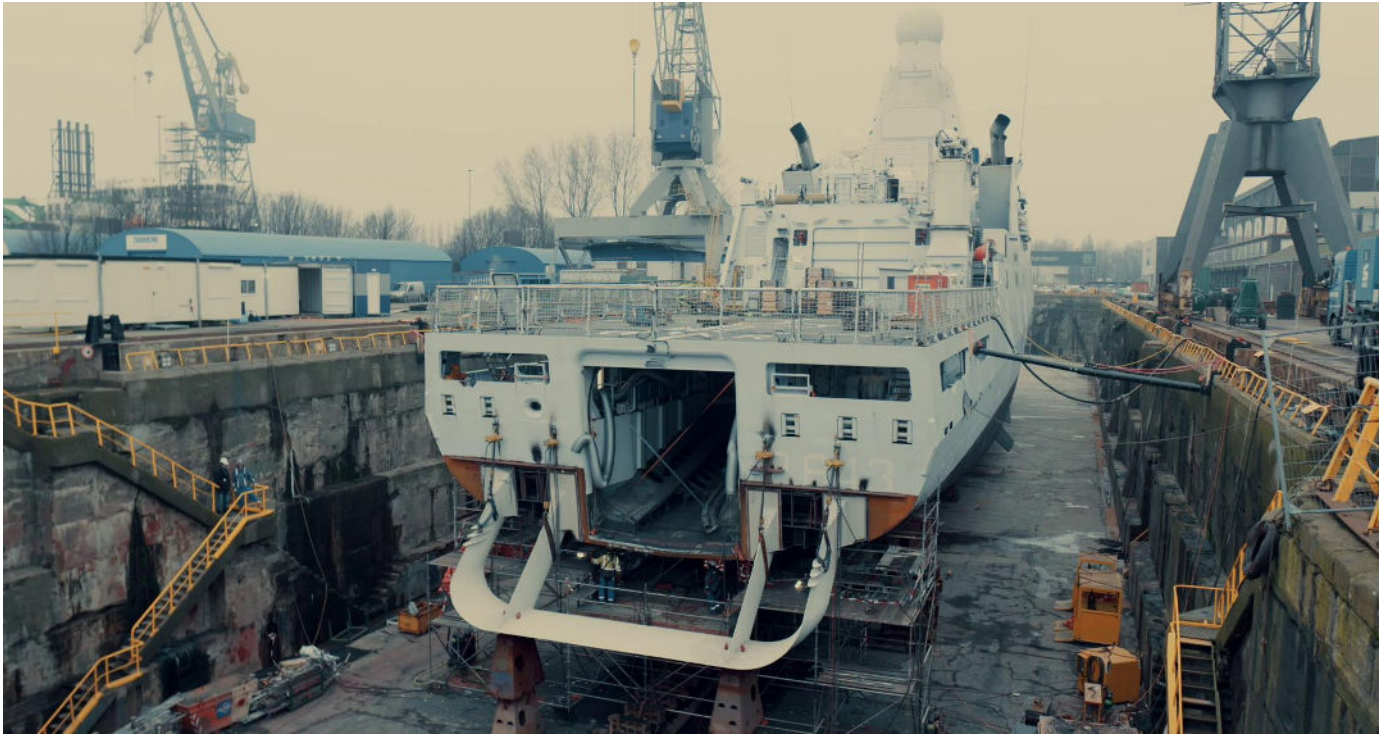
Figure 5 - Hull Vane® installed
