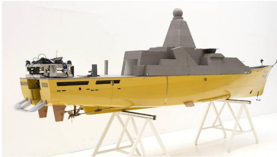
Figure 3 - Tank test model Holland-Class © Dutch Ministry of Defence
