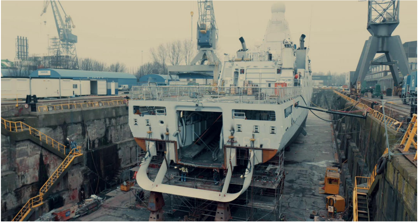
Figure 4 - Hull Vane® installed
