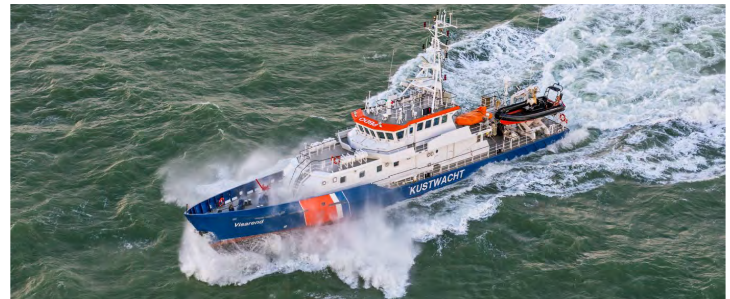
Full power (22.7 knots), with Hull Vane®
