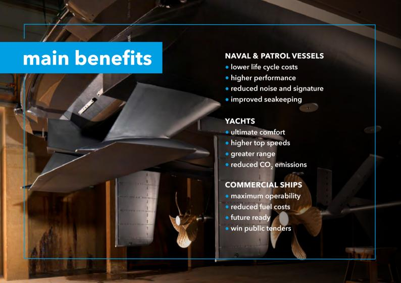
The Hull Vane® is a hydrodynamic wing attached to a ship's stern. It's positioned so that it suppresses the stern wave and angled so that the flow of water around it generates forward thrust. This also reduces overall resistance and dampens pitching, heaving and rolling when sailing through waves. Depending on vessel suitability and factors such as its length, speed and hull design, a Hull Vane® can reduce fuel consumption by anywhere between 5 and 26%.
