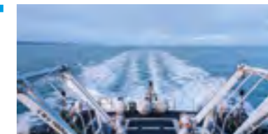
Wave profile at 15 knots without Hull Vane®
