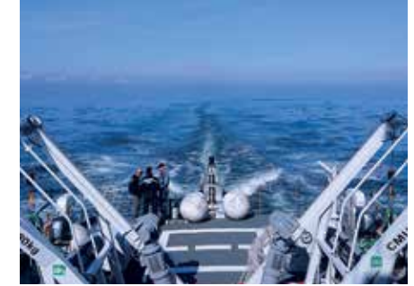
Wave profile at 15 knots with Hull Vane®
