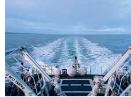
Wave profile at 15 knots without Hull Vane®
