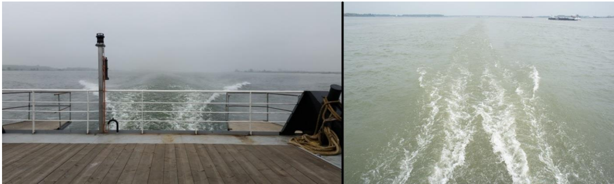
Fig. 4. Comparison of the wave profile of the 55 metre supply vessel without Hull Vane ® (left) and with Hull Vane ® (right) at 13 knots, as seen from the aft deck during sea trials.
