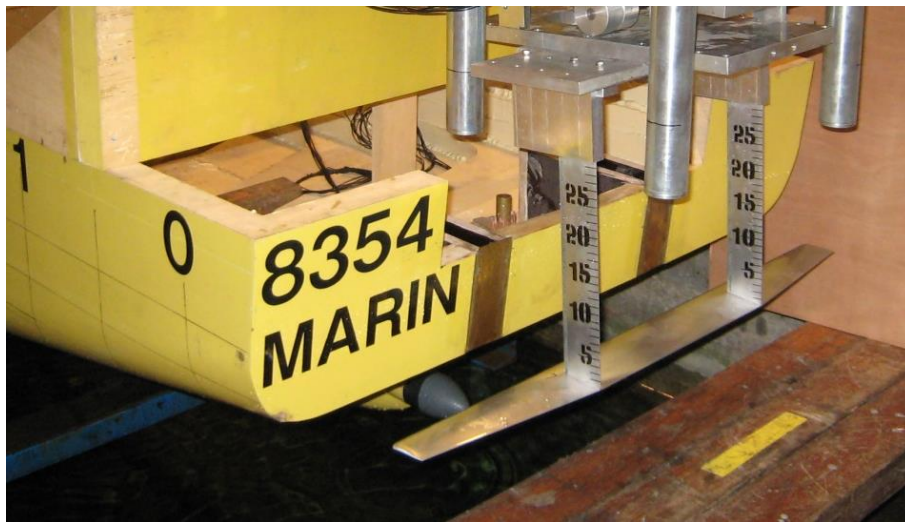
Fig 7. One of three Hull Vanes ® as tested on a model of a 169 metre container vessel.
