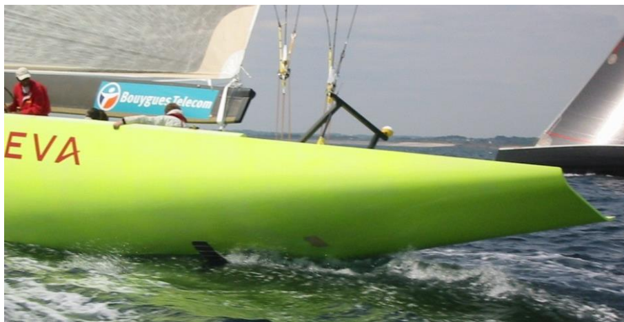
Fig. 1. The second application of the Hull Vane ® , on the 2003 IACC yacht Le Defi Areva .
