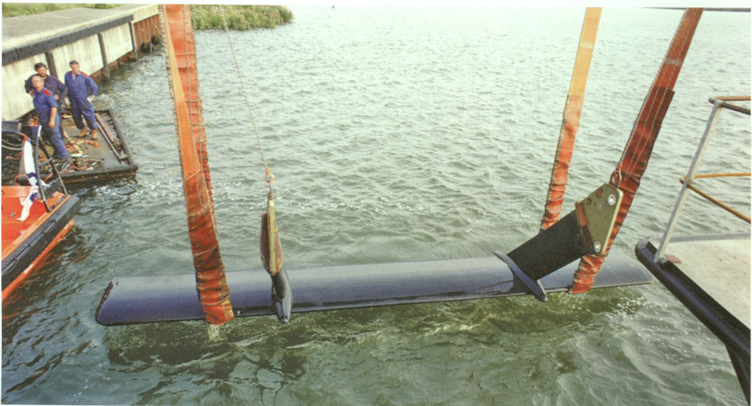
The Hull Vane can be installed on newbuild vessels or retrofitted to existing vessels
