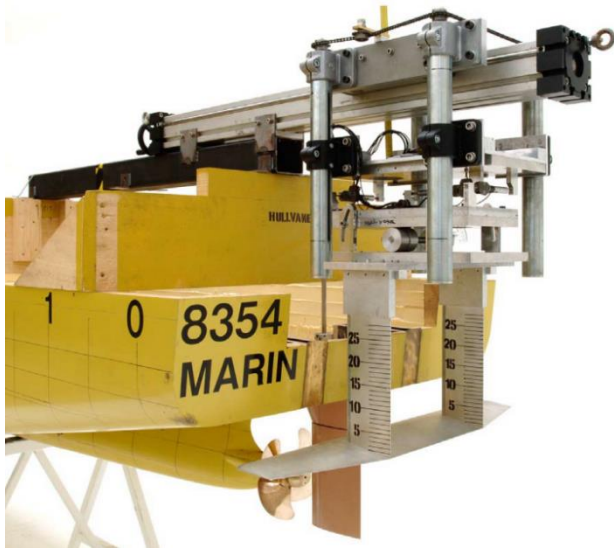
Figure 1: Tank test setup with Hull Vane.
