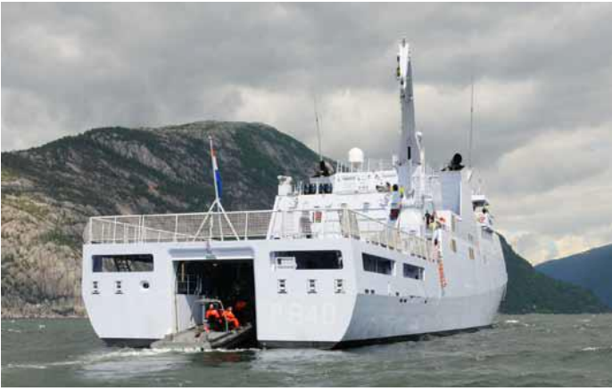
Figure 7: Slipway arrangement of the Holland Class OPVs
