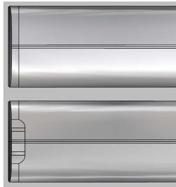
Figure 10: Bottom view of stern: benchmark vs. modified
