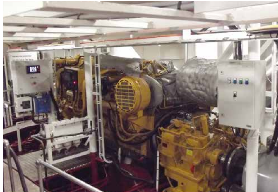
Two Caterpillar diesel engines are connected directly or indirectly to the propellers
