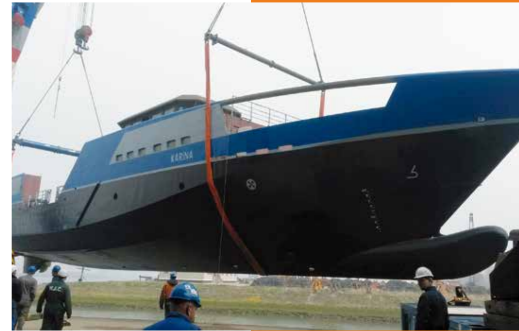
As the design of the FSIV allows for lifting it with a crane, docking has become almost obsolete
