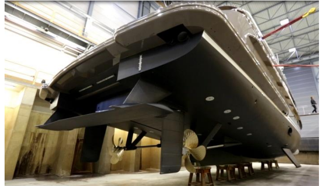
Figure 2: Application of the Hull Vane ® on the 42 metre motor yacht Alive .
