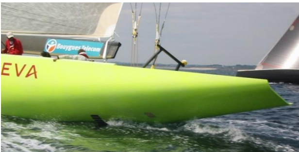
Figure 1: The second application of the Hull Vane ® , on the 2003 IACC yacht Le Defi Areva .
