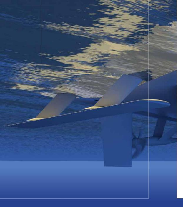
Hull Vane® — An energy saving and (passive) seakeeping device for medium-speed and fast displacement vessels
