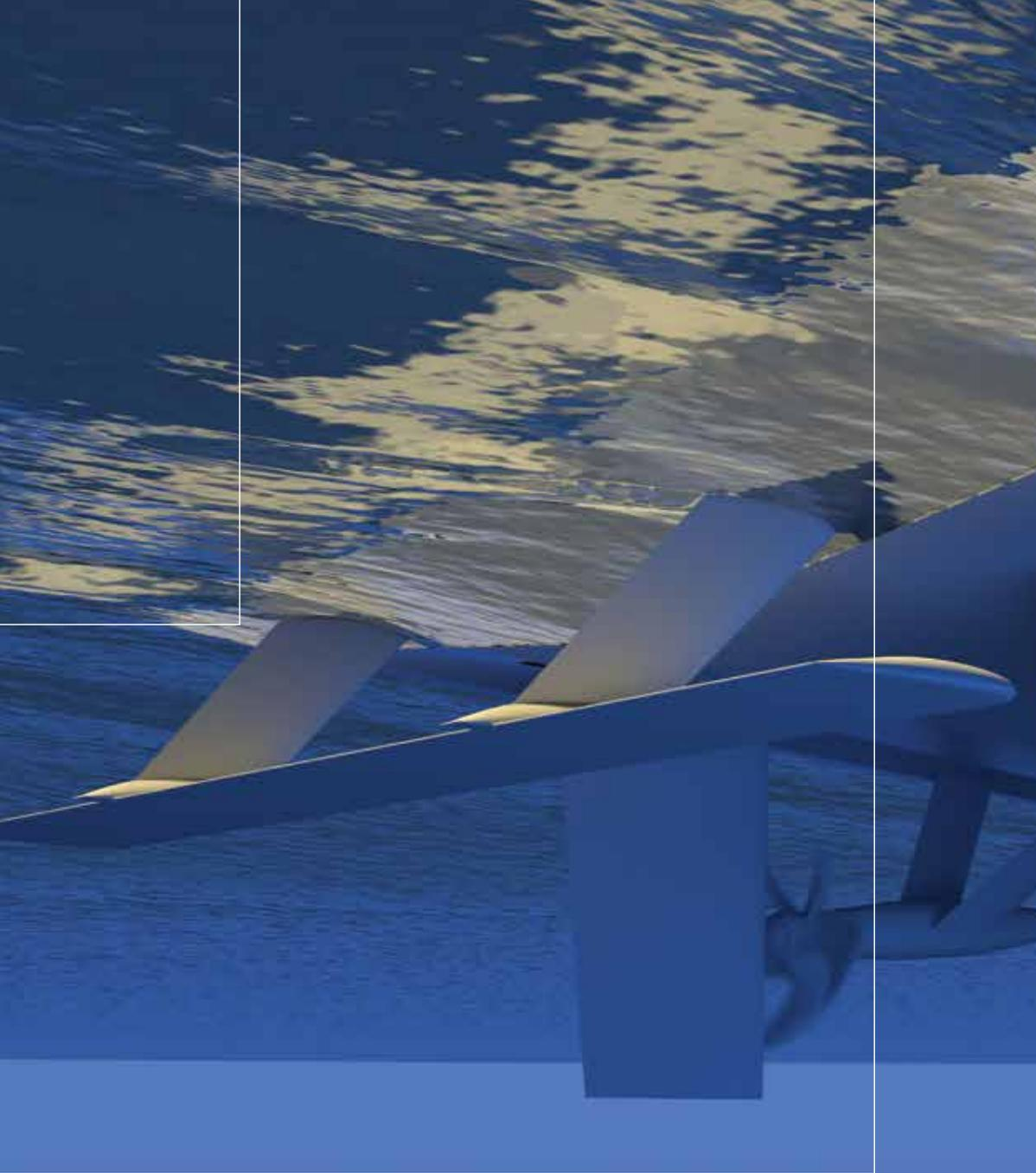
The Hull Vane<sup>®</sup> is a fuel saving device in the form of a fixed foil, located below the stern of a ship.
